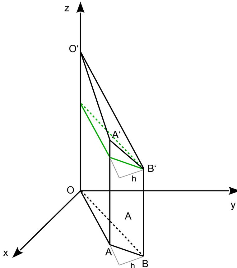
$$\begin{array}{lll} O(0 \mid 0 \mid 0) & A(x_A \mid y_A \mid 0) & B(x_B \mid y_B \mid 0) \\ O'(0 \mid 0 \mid h_O) & A'(x_A \mid y_A \mid h_A) & B'(x_B \mid y_B \mid h_B) \end{array}$$
